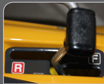
Easy cruise control style ground speed control.
