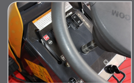
DASH MOUNTED DIFF LOCK AND 4WD CONTROLS.
