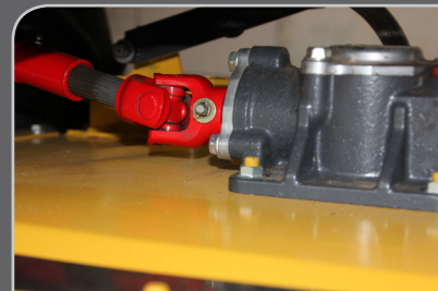
SUPER TOUGH SHAFT DRIVEN GEARBOX WITH ADJUSTABLE DISCHARGE DECK.
