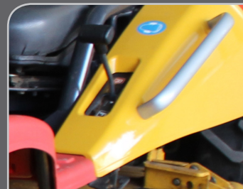
Easy cruise control style ground speed control.
