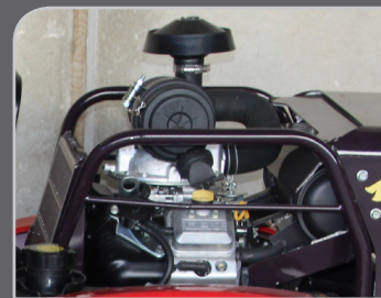
21HP V-Twin Vanguard Engine.
