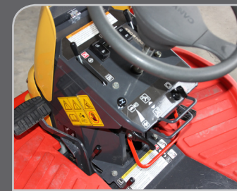
Dash mounted Diff Lock/dual range 2WD/4WD controls.
