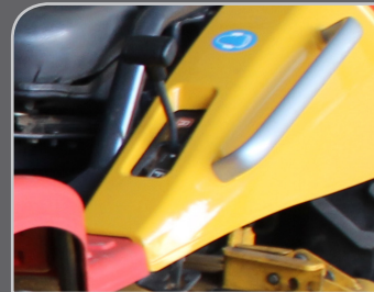
Easy cruise control style ground speed control.
