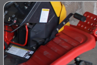
FOOT PEDAL HEEL/TOE FORWARD REVERSE.
